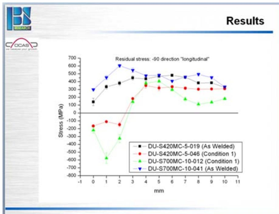
Figure 5: Residual stress measurements: Comparison of S420 and S700
