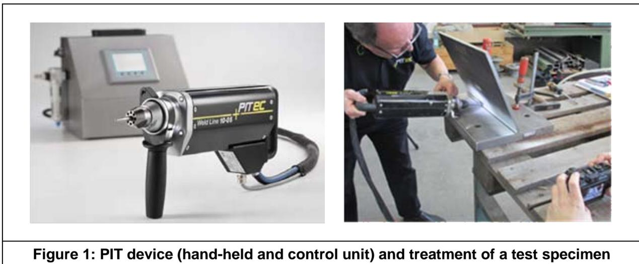
**Figure 1: PIT device (hand-held and control unit) and treatment of a test specimen**
