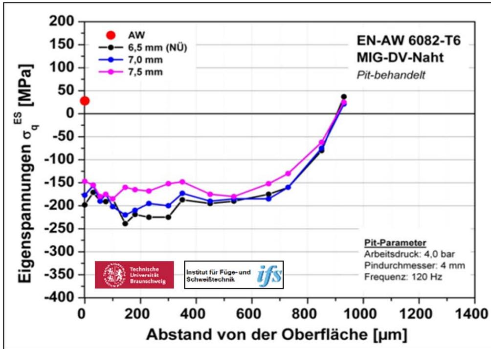
Figure 4: Residual stress measurements: Aluminum joints
