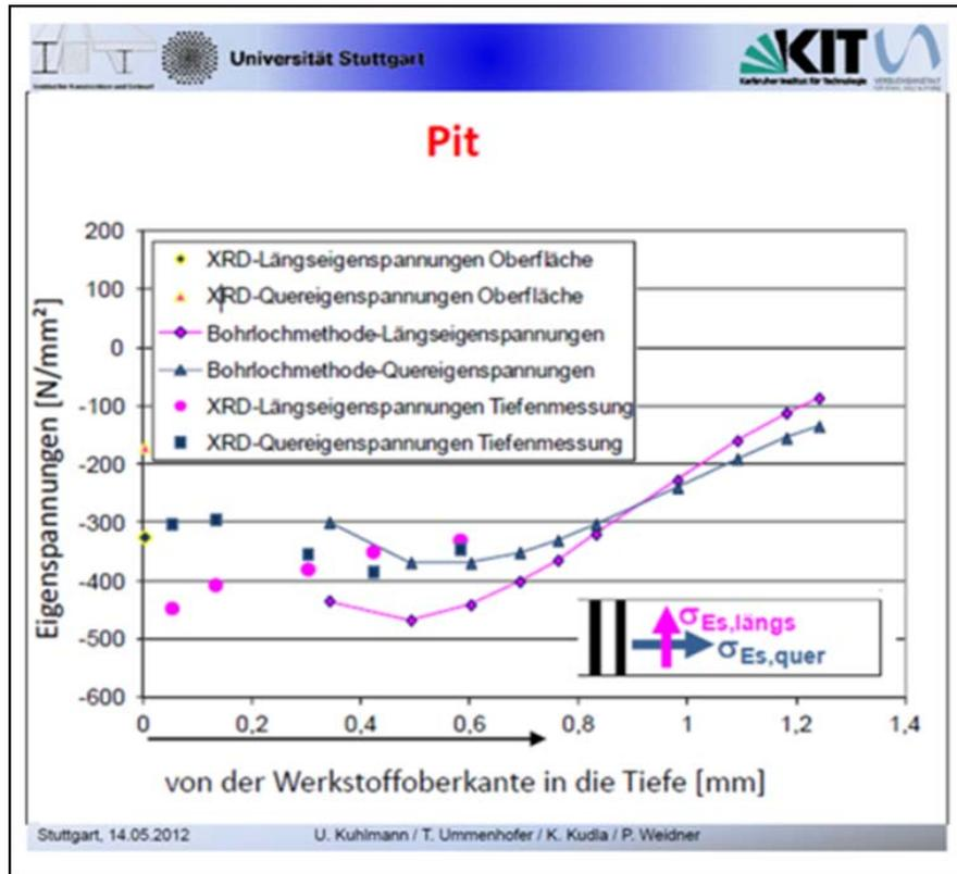
**Figure 6: Residual stress measurements: Comparison of X-ray diffraction and hole drilling method**
