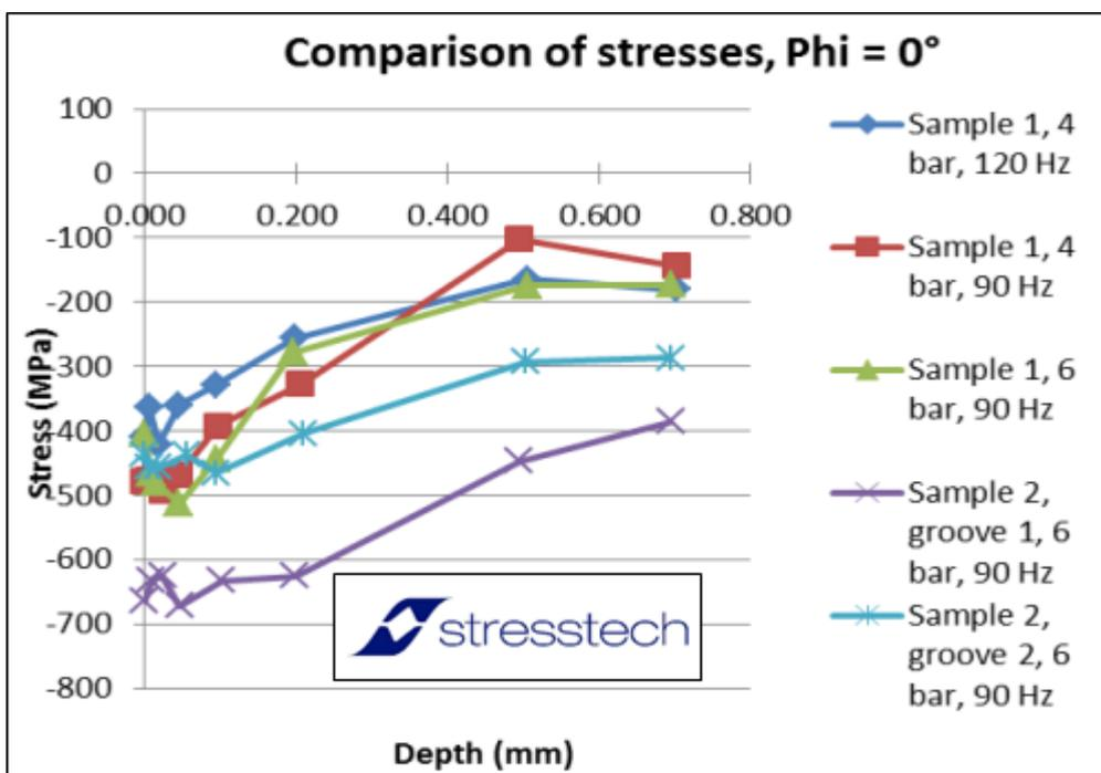
**Figure 3: Residual stress measurements: PIT treatment with different parameters**
