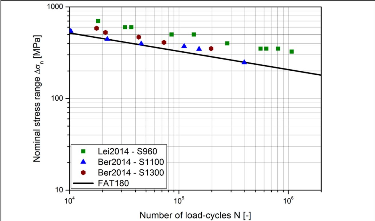
Figure 17 — Longitudinal welds with  $950 < f_y$
