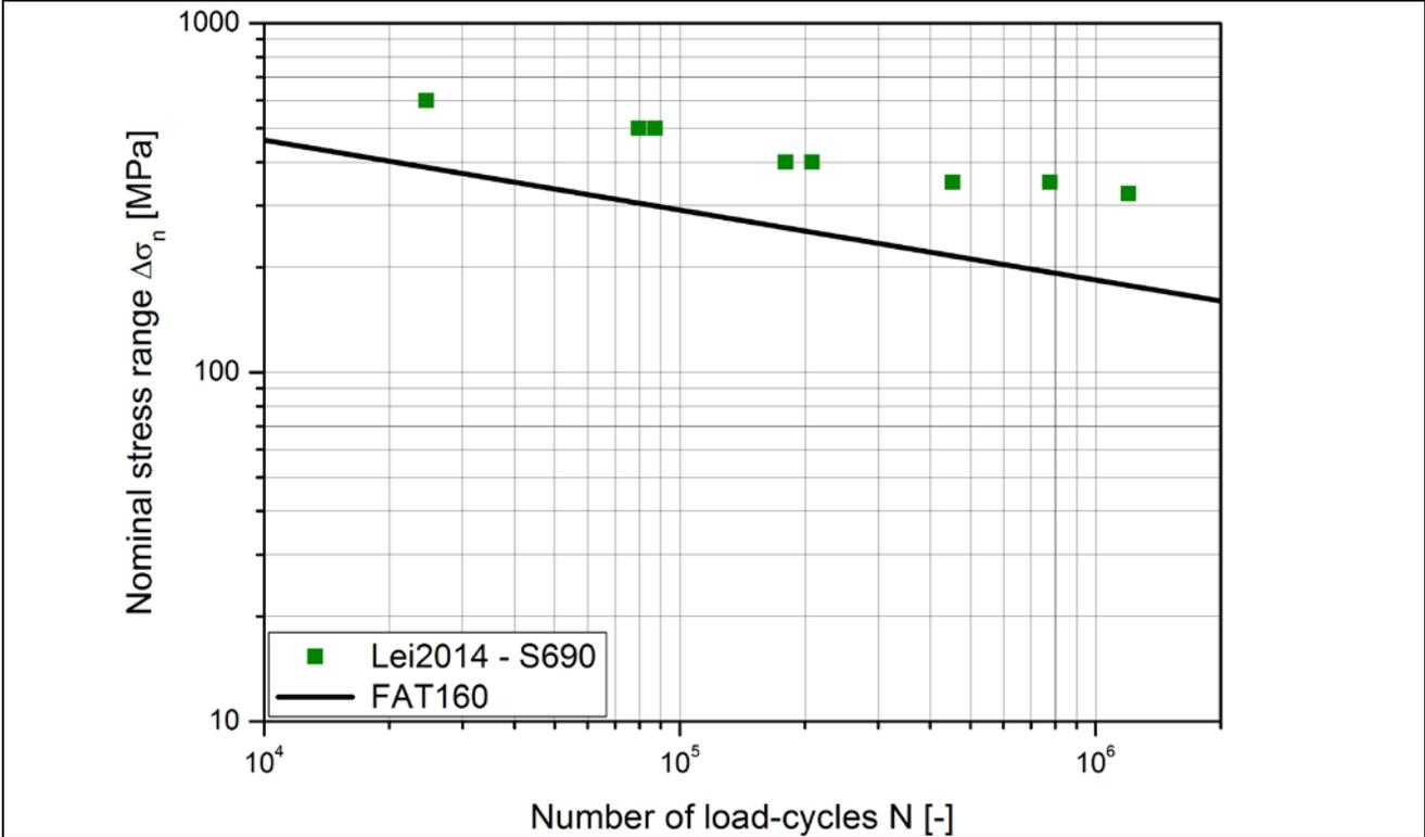
Figure 12 — Transverse welds with  $550 < f_y \leq 750$
