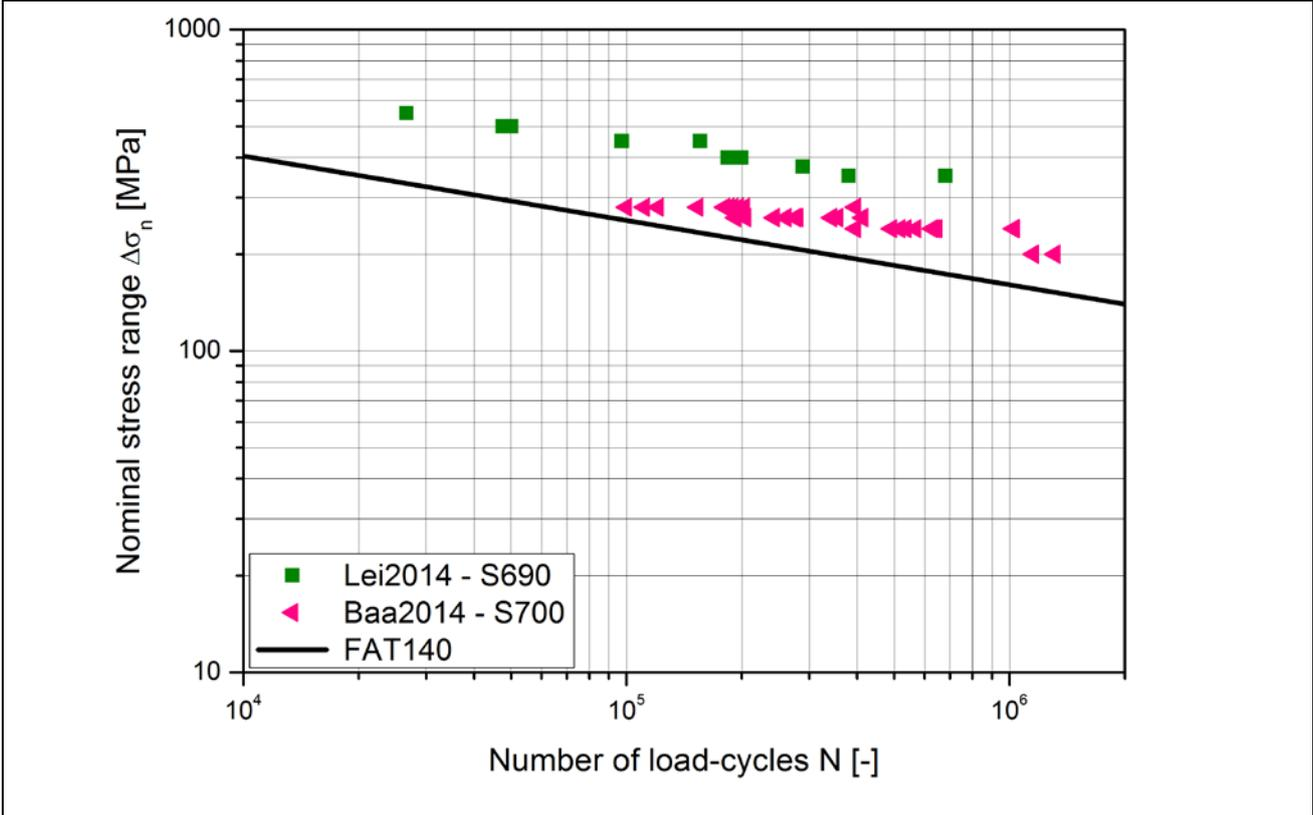
Figure 16 — Longitudinal welds with  $550 < f_y \leq 750$
