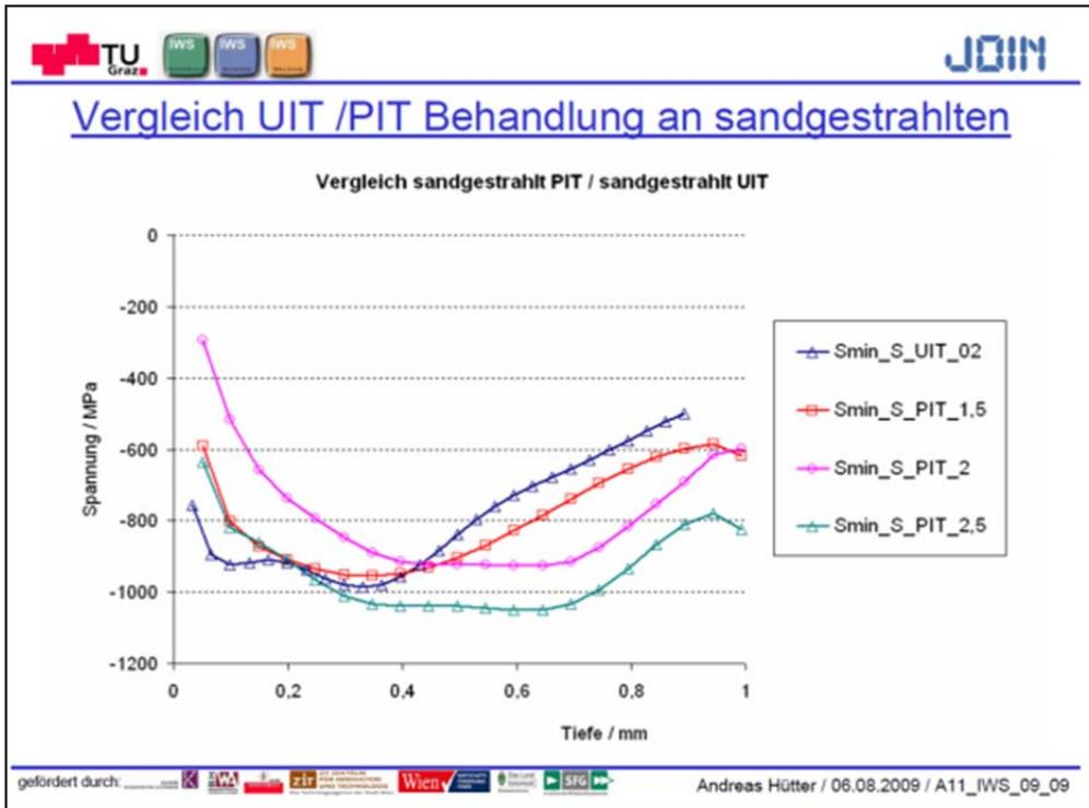
**Figure 2: Residual stress measurements: Comparison of UIT and PIT**
