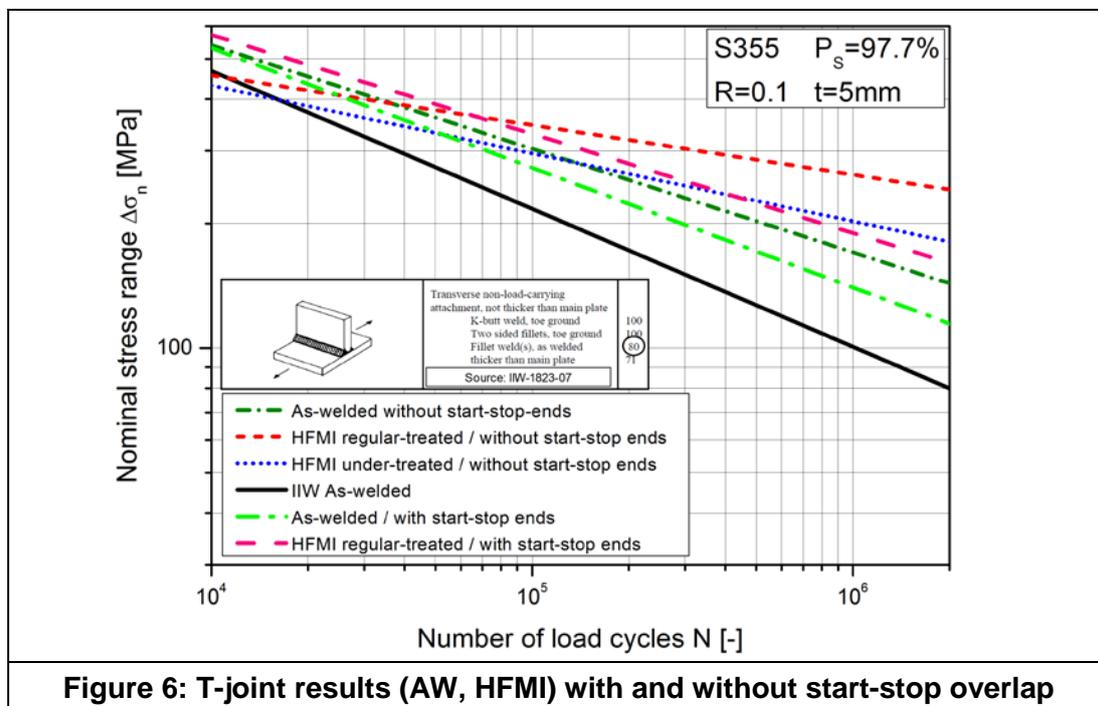
Whereas the geometric heterogeneity of the start-stop end region has a significant effect on finite fatigue strength, a regular-treated HFMI process is capable to enhance the both S/N-curves. Proper HFMI-treatment leads to a unification of, comparably small, weld process manufacturing effects into a single design curve.
