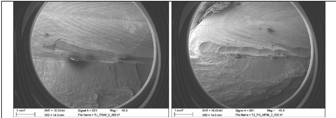
**Figure 7: Fracture surface of T-joint with start-stop overlap (as-welded versus regular-treated HFMI condition)**
