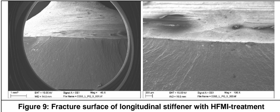
**Figure 9: Fracture surface of longitudinal stiffener with HFMI-treatment**
