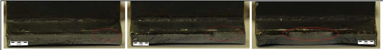
**Figure 3: HFMI-process study of fillet welds on T-joints (under-treated, regular-treated, over-treated)**
