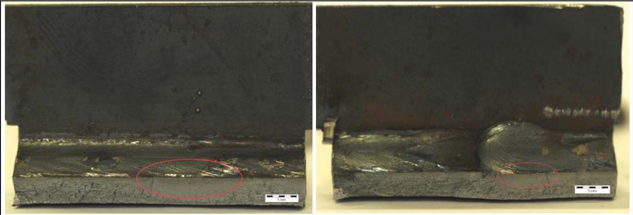
**Figure 1: Fillet weld in as-welded condition (fillet; start-stop overlap); no HFMI**
