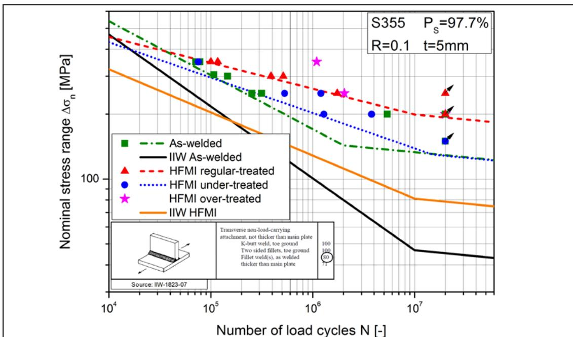
**Figure 4: Non-load carrying transversal attachment results in as-welded vs. HFMI-treated condition (both without start-stop ends)**
