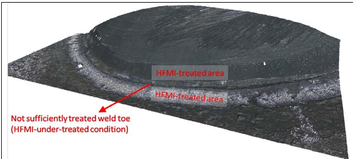
**Figure 2: Spatial laser scanning of under-treated HFMI weld toe region (exemplified for a longitudinal attachment sample)**
