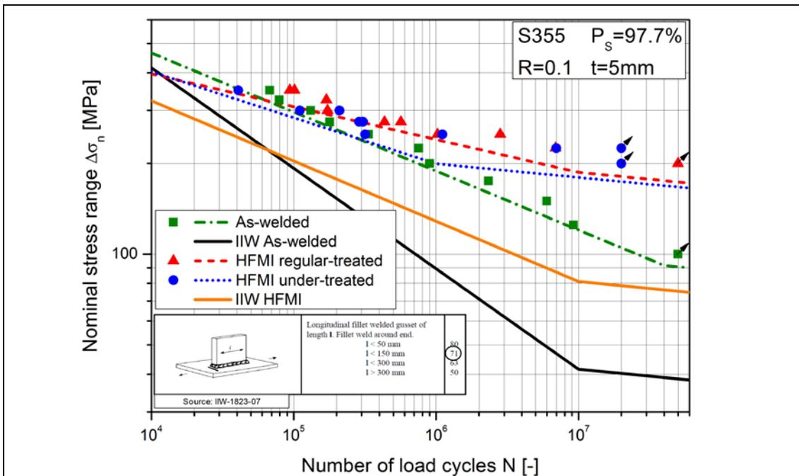
**Figure 8: Longitudinal stiffener fatigue strength results (as-welded vs. HFMI process settings)**
